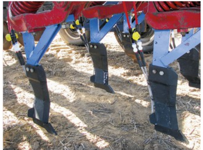
Bent-leg openers, such as this South African prototype RT Blade, could potentially deliver quantum leaps forward in no-till seeding.
