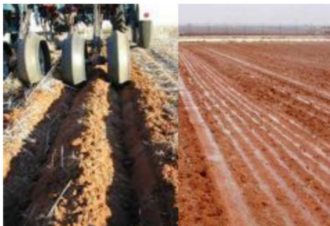
Figure 28. This Australian press wheel has a wide angle creating a large and stable furrow surface shape (right) which can 'harvest' water during small rainfall events and concentrate it near the seed (left).
