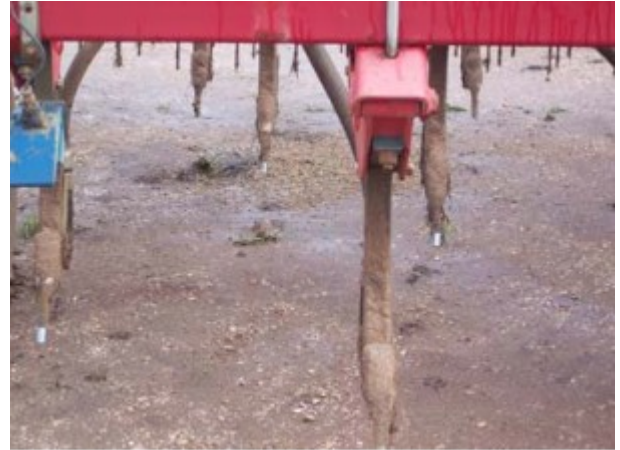
Photo : 12mm knife points are used on flexicoil tines
